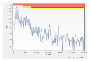
linear scale may be adequate in cases where components are all nearly the same size, but in case of machinery vibration, incipient failures in parts such as bearings produce signals with very small amplitudes.
