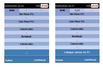
Pressing continue measures an initial spectrum of system and then the initial unbalance value will be measured automatically, press continue again and this value is saved and indication to place the test weight appears.
