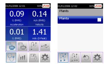
In Configuration mode, activate "Connect to PC" option. The message "Connect the equipment to the PC" will appear; at that time connect equipment using the USB cable provided, then proceed to load a route as described in the Machinery Control Software manual. After this disconnect USB cable (always perform a safe disconnect, using the standard Windows procedures from PC) press
