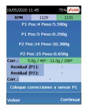
For rotor, remove test weight from plane 2, place correction weights in each plane, place sensor on plane 1 and start rotor, pressing continue will show vibration value obtained on plane 1, press continue and place the sensor in plane 2, pressing continue will show the value obtained in plane 2.
